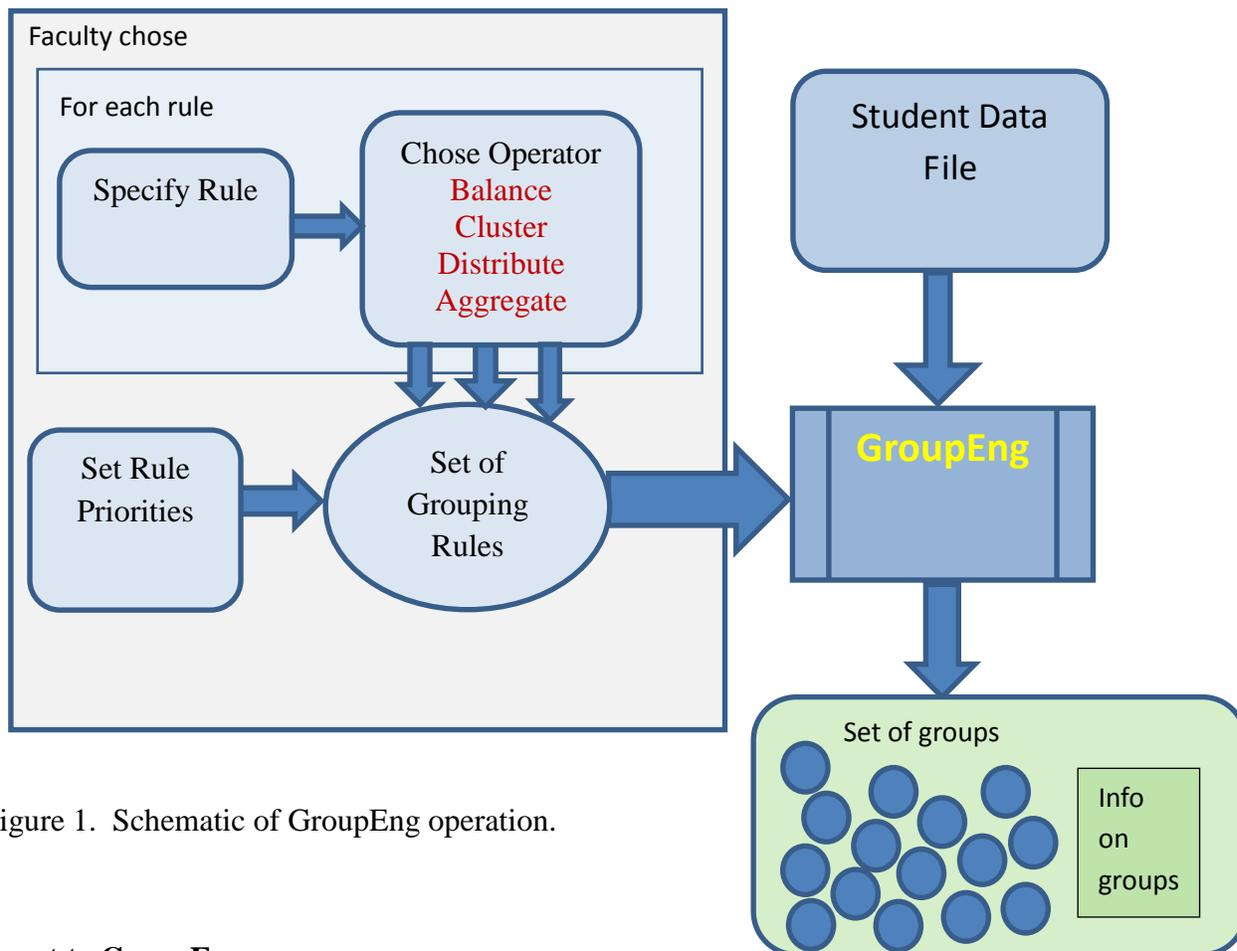
Figure 1. Schematic of GroupEng operation.
